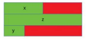
• The red portion represents the padding added for data alignment and the green portion represents the struct members. In this case, **x** (int) is followed by **z** (double), which is larger in size as compared to **x**. Hence padding is added after **x**. Also, padding is needed at the end for data alignment.
